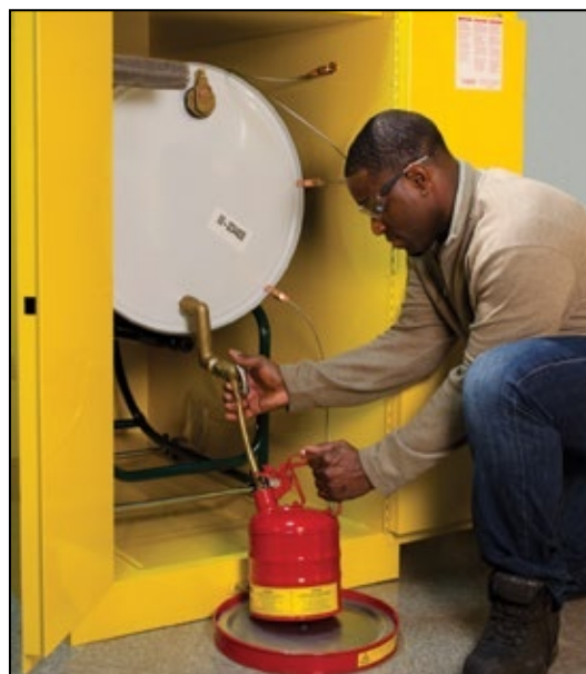
Use proper grounding techniques when dispensing flammable liquids
