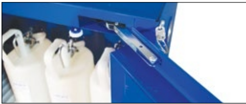
Encased self-closing mechanism provides obstruction-free access to top shelf space. Fusible link melts at 165°F (74°C) to automatically close door(s) under fire conditions.
