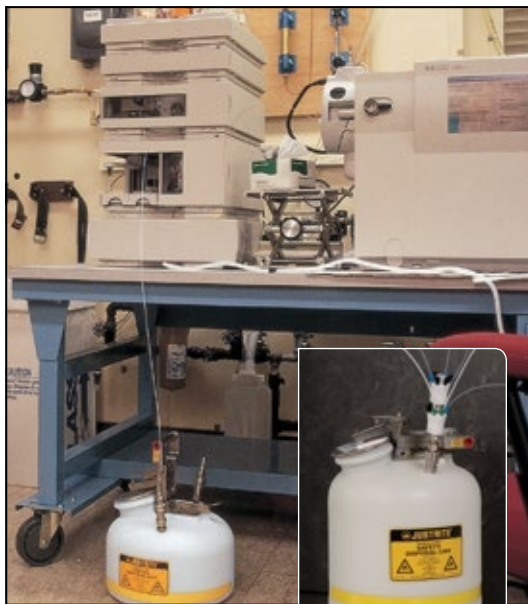
Manifold kit provides a convenient, cost effective way to collect waste from multiple HPLC machines.
