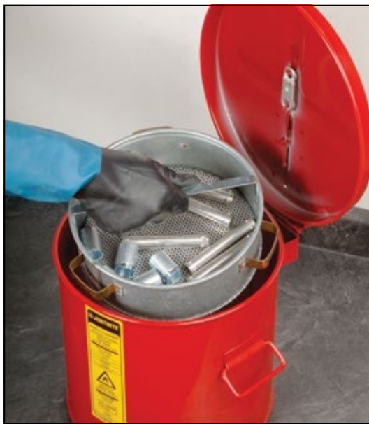
Clean small parts by immersing basket into solvent.
