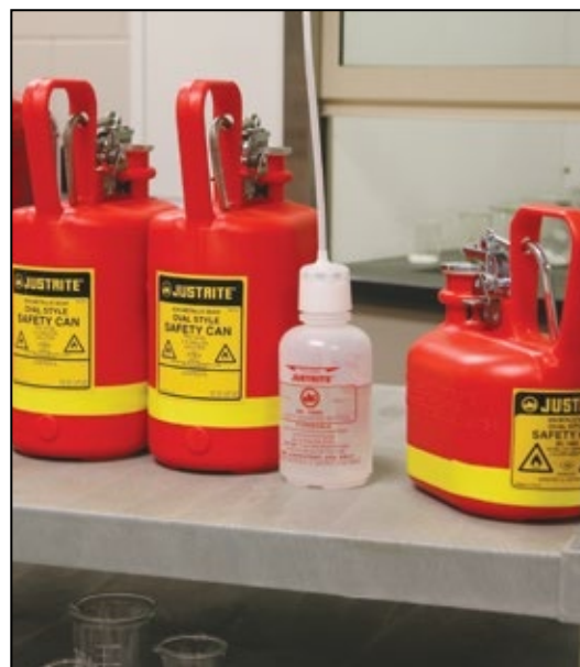
Use smaller capacity safety cans with flame arresters to safely dispense and store chemicals found in laboratories.
