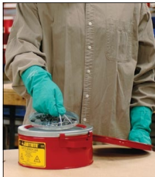
Clean small parts by pushing down dasher plate and agitate in cleaning solvent.
